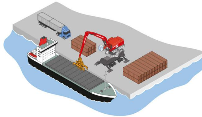
Our material handlers are all-weather designed, allowing the port to carry out non-stop work. Rigid boom is immune to swinging and wind compared to traditional harbour cranes making the operations fully controllable all the conditions.
